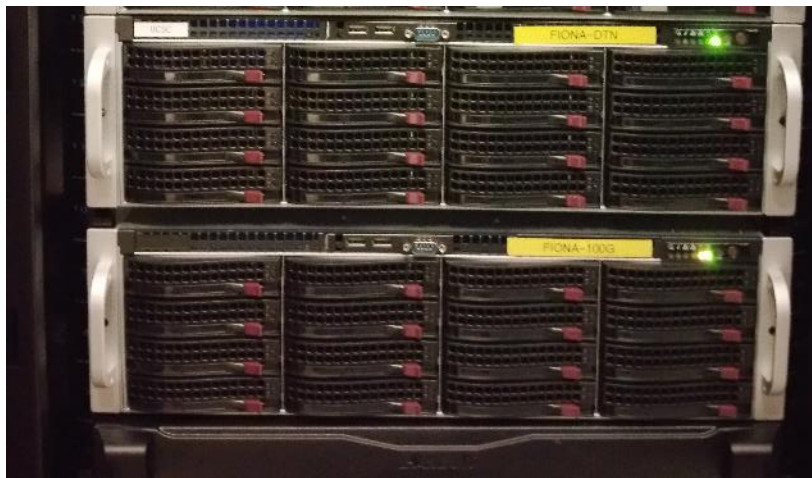
Two FIONA DTNs at UC Santa Cruz: 40G & 100G Up to 192 TB Rotating Storage
