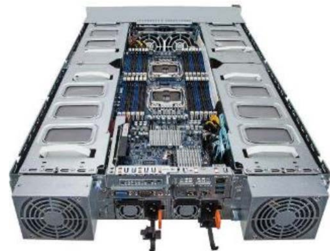
Add Up to 8 Nvidia GPUs Per 2U FIONA To Add Machine Learning Capability
